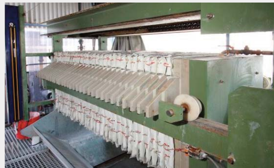
10m 3 fully automated dewatering sludge filter press Installation
