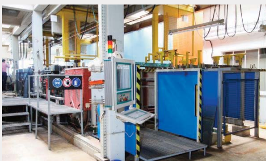
Copper/nickel/chrome plating plant to suit various base metals
