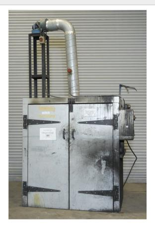
Stock No Model Internal Size (WxDxH mm) Max Temp External Dimensions (WxDxH mm) OS1231 Drying cabinet 1500 x 750 x 1700mm 250°C 1950 x 1200 x 2400mm
