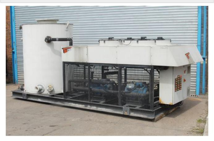
Stock No Manufacturer Model Year of Manufacture Serial Ave. cooling capacity Other Info Weight (kgs) External Dimensions (WxDxH mm) CQ409 Industrial Cooling Systems (ICS) TED 92086 Sept 2000 TEC 452 172kW Refrigerant R22 950kg 1620 x 4800 x 2140mm high (with tank)
