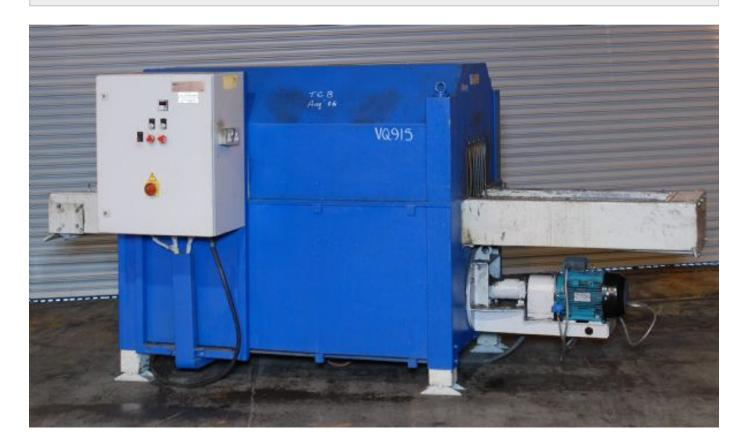
Stock No Manufacturer Model Year of Manufacture Capacity Type Other Info VQ915 Walther Trowal BFHL350 2002 600I Vibratory Process Bowl Continuous parts dryer
